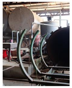
Treatment of wood with impregnation (vacuum-pressure-vacuum or VPV method) is an option for customers needing extra termite protection. We use "Tim-bor," a salt-based product that is safe for people and the environment to preserve the Teak and ensure that every surface of the wood is deep and well preserved.
